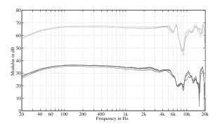
**Figure 6:** Equalization response for two subjects using the black filter from Fig. 5, also for the Sennheiser HD600 headphone. The dark gray curve is shifted -30 dB for clarity.
