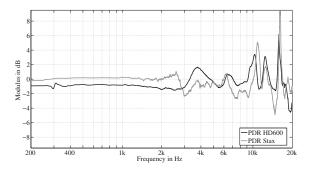
**Figure 8:** Pressure division ratio for headphones Stax SR Lambda and Sennheiser HD600. Average of eight HpTF measurements made with the help of a mounting devide to reduce high frequency variability and HRTF measured for five different directions.
