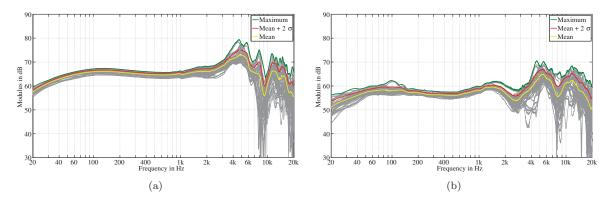
**Figure 4:** Individual HpTF measured at 15 subjects (4 repetitions). Subjects should place the headphone at its most comfortable fit. Left speaker of (a) Sennheiser HD 600 and (b) Stax SR Lambda.
