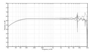
**Figure 1:** Frequency response of a headphone equalized with a filter designed from the average of four HpTF and no equalization below 100 Hz.
