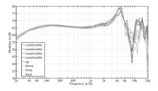
**Figure 3:** HpTF of a single subject measured four times with comfortable fit and at four extreme positons with the Sennheiser HD600 headphone.
