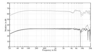
Figure 7: Equalization response for two subjects using a individual filter. The light gray curves were generated with the filter shown in Fig. 5. Dark gray curve is shifted -30 dB for clarity.
