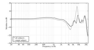
Figure 5: Equalization filter for the Sennheiser HD600 headphone obtained by inverting  $\mu + 2\sigma$  from 15 subjects (black) and of a single subject (gray).
