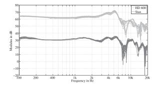
Figure 2: HpTF of two open-type headphones measured with a dummy head. 18 fittings are shown for Sennheiser HD 600 (light gray) and Stax SR Lambda (dark gray, values shifted -30 dB for clarity).
